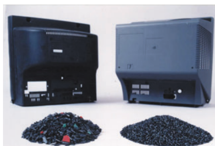
(left) Used TV cabinets and plastics before treatment (right) Recycled TV cabinets and plastics after treatment
