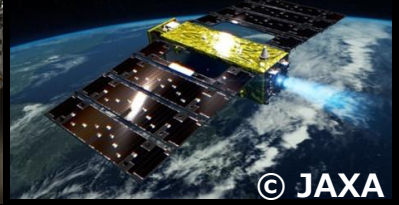
2017 "SLATS" Exposure testing of materials in very-low earth orbit (altitude : 160km)
