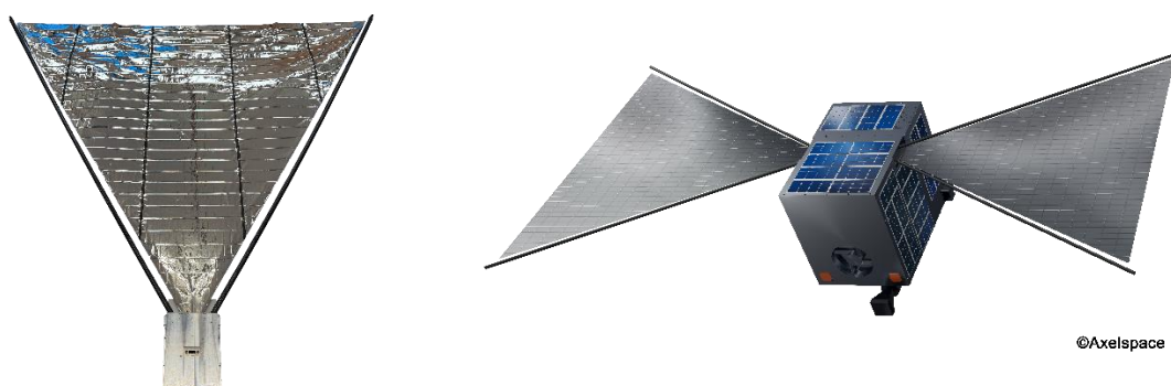
A photograph of D-SAIL (left) and a conceptual image of its membrane deployment on GRUS-3
